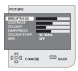
You can select the desired title to be processed from this menu. You can select the desired setting by pressing the **Up/Down** movement buttons and adjust their levels with **Right/Left** movement buttons. You can adjust **BRIGHTNESS**, **CONTRAST**, **COLOR** and **SHARPNESS** levels as you desire. The changes you have made in the picture settings will be stored in the memory without requiring any other operations.
